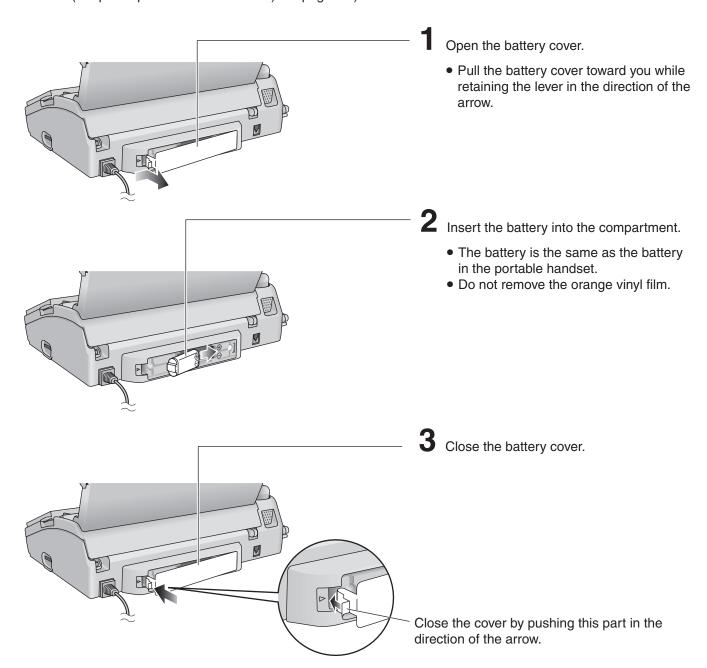
• The charging time for the battery of the main unit is about 10 hours.
