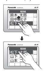
While touching the screen when  $\boxed{\phantom{a}}$  and  $\boxed{\phantom{a}}$  are displayed, move (flick) your finger in the direction of the name that you wish to display.
