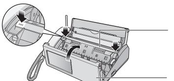
If the ink film is slack, tighten it by winding this gear (orange).
