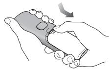
2 Insert the battery into the compartment and close the battery cover.
