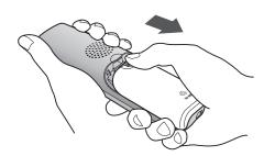
2 Insert the battery into the compartment and close the battery cover.
