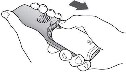
**2** Insert the battery into the compartment and close the battery cover.
