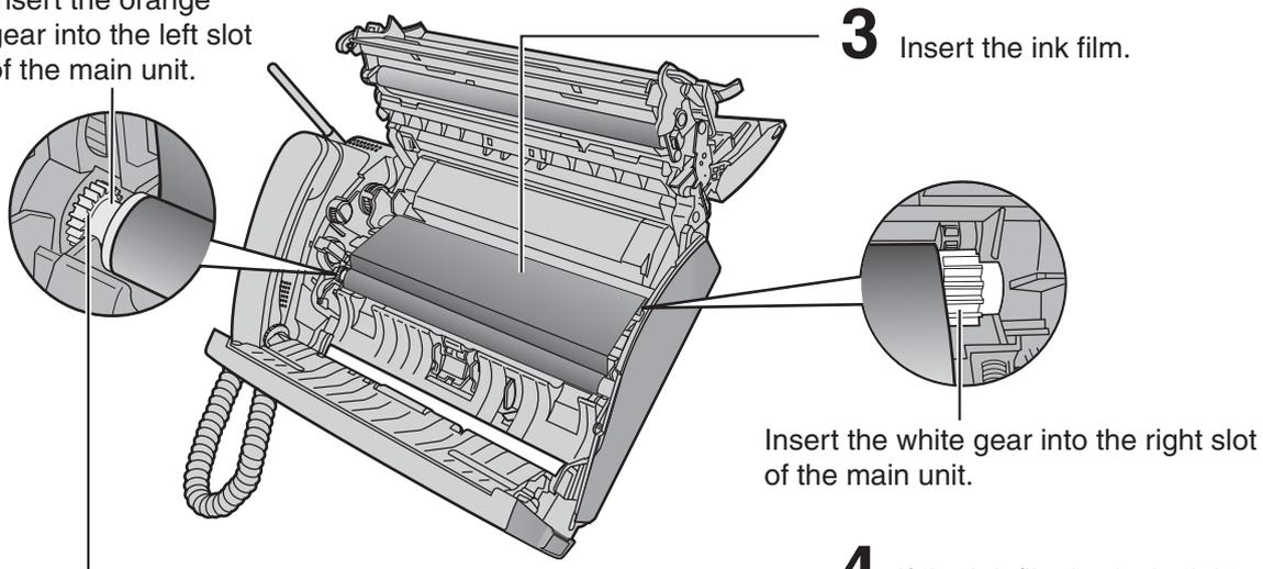
**4** If the ink film is slack, tighten it by winding this gear (orange).
