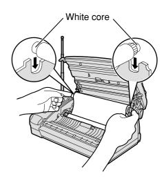
5 If the ink film is slack, tighten it by winding the "T" shaped gear.
