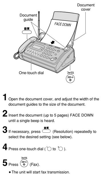
Select the desired resolution according to the type of document, by pressing  $\bigcirc$  (Resolution).
