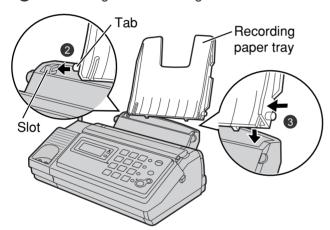
2 Insert the recording paper into the recording paper tray.
