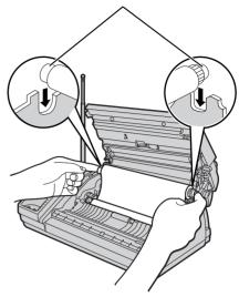
If the ink film is slack, tighten it by winding the "T" shaped gear.
